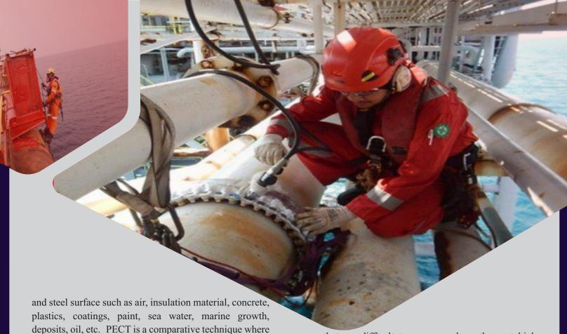
and steel surface such as air, insulation material, concrete, plastics, coatings, paint, sea water, marine growth, deposits, oil, etc. PECT is a comparative technique where the percentage variations measured on the specimen are compared with a calibration value which is always assumed to be the full wall thickness.
