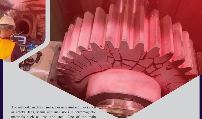
advantages of magnetic particle inspection is that it can give an immediate indication of defects and
