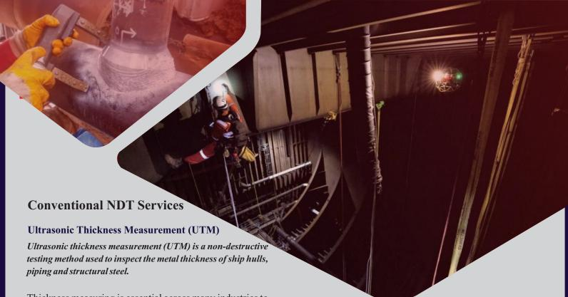
Thickness measuring is essential across many industries to monitor corrosion, erosion and damage. Ultrasonic thickness measurement (UTM) is commonly used and the method can be applied to a wide range of structures and components that includes ship hulls, piping, pressure vessels and structural steel.
